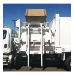
Lowest industry dump height at just 14' with a lift capacity of 4200 lbs.
